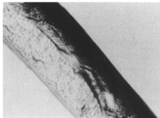
Figure 4. A microscopic photograph of a cross-section of a composite membrane (NEOSEPTA CM-1 and polypyrrole; polymerization time: 4 h).
